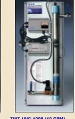
TWT-UVC-1200 (12 GPM) Ultraviolet Disinfection/Purification System Mounted on St/St Frame with Manual Shut-Off Valves Alarm • UV Monitor and Automatic Solenoid Valve • Size: 20"W X 44"H 10"D Available 120V/60 Hz or 230V/50 Hz
